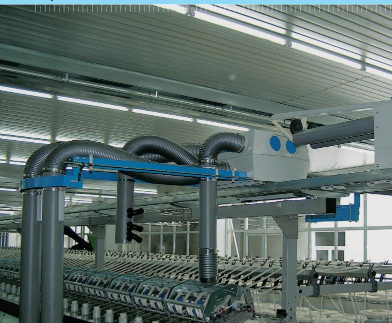
Automatic travelling cleaner for roving, spinning, winding, twisting and for warping and weaving
