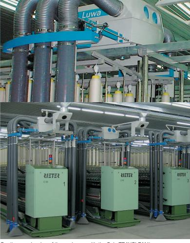
Continuous cleaning of the work area with the Spin TRAVCLEAN® considerably increases the machine's efficiency. Higher quality of the yarn will be assured due to the reduction of tread breakage and less fiber fly.
