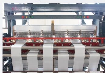
Solution for filter tube braiding (16cm/6 tapes)
