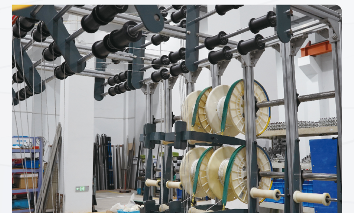
Tape tension control Electronic let-off system
