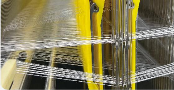
By using jacquard leno heddle , to control the single or multiple warp yarn to cross over and tie up another single or multiple warp yarn, thus create the pores on the cloth surface, to achieve the function and effect of breathable or hollowed out on the shoe upper or other fabric
