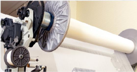
Patent protected unique leno warp tension control system, can precisely control each individual cross weaved warp yarn controlled by leno heddle, no matter what kind of jacquard patten, in any position of the fabric, could achieve the smoothest cross movement of the warp yarn, achieved the free weave of jacquard leno design
