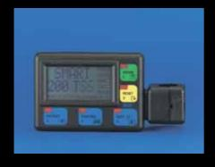
The "touch light" function allows for the rapid and precise use of the optic key in the different procedures. Bright (red and green) LEDs are used for control condition and alarm signalling.
