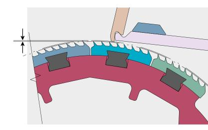
Several options for the point density of the top comb (23, 26, 29, 32 points/cm). Marzoli offers a top comb which automatically cleans its points through a jet of compressed air (option).
