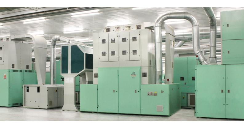
Four or eight blending chambers with additional tuft blend through suction in the blending channel and production rates up to 1,600 kg/h.
