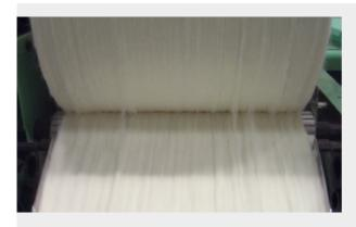
Standard lap winders: irregularity of the superimposed cotton layers
