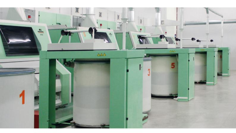
Marzoli's C701 card has been specifically designed to achieve a superior tradeoff between quality and productivity in processing any type of fiber. This has been possible thanks to the great number of innovations in some specific areas of the machine.
