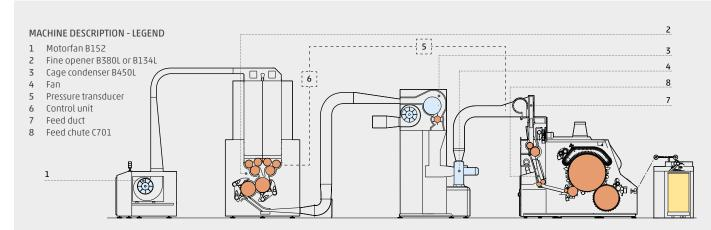
The B153L delivers up to 800 kg of material per hour to the cards. The material is sucked from the previous machine by a B450L cage condenser, which removes
