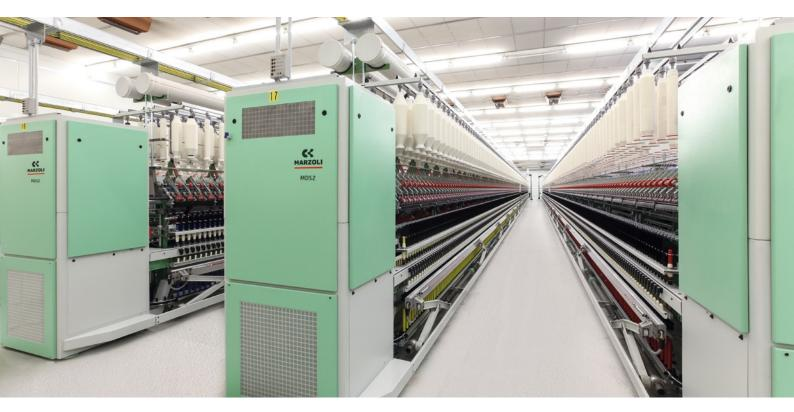
Marzoli ring spinning frames, the MDS2 and the MP1N, are fully electronic machines with independent drives for spindles, ring rail and drafting system.
