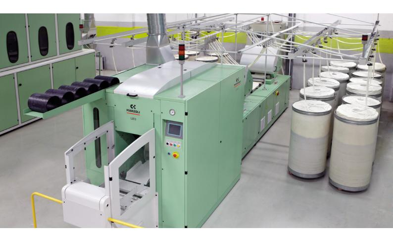
The LW3 lap winder represents the best technology for quality and productivity. The innovative design of its lap formation area with 4 calenders and a compacting cylinder to avoid expansion of the wound layers allows to reach an average speed of 190 m/min. This, together with an automatic doffing system of only twenty seconds,
