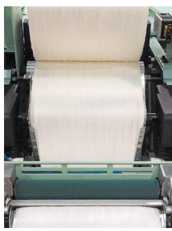
Standing pendulum movement of the nipper to maintain minimum and constant distance between the jaws and the circular comb throughout the combing cycle. Top quality of circular combs with 4 sectors (combing angle of 90°) or 5 sectors (combing angle of 112°) with progressive point density, specifically designed to process thick batts at high speed.
