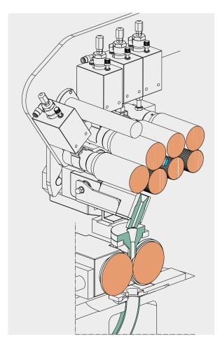
After the condenser, a calender compacts the sliver and scans its mass with calculation of sliver count deviation and CV%.
