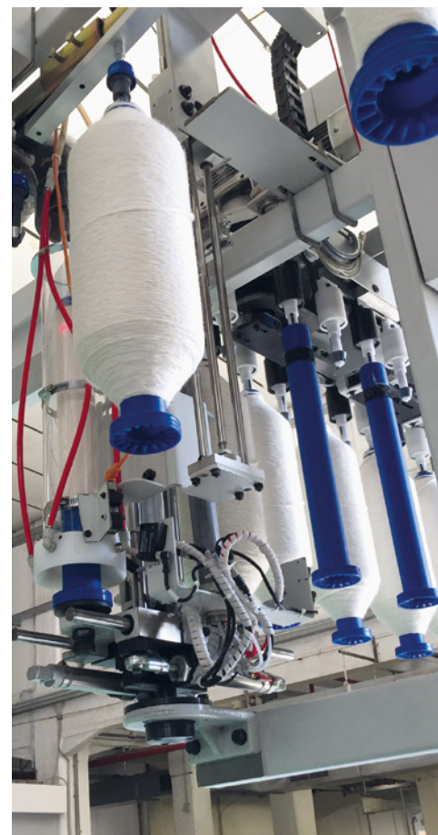
IBC - bobbin stripper integrated on the exchanger
