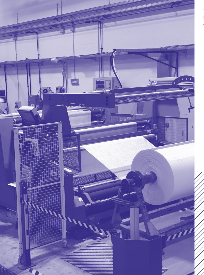
+ 3000 set-up models around the world The Set-Up model allows feeding the fabric non-stop into the traditional printing machines.
