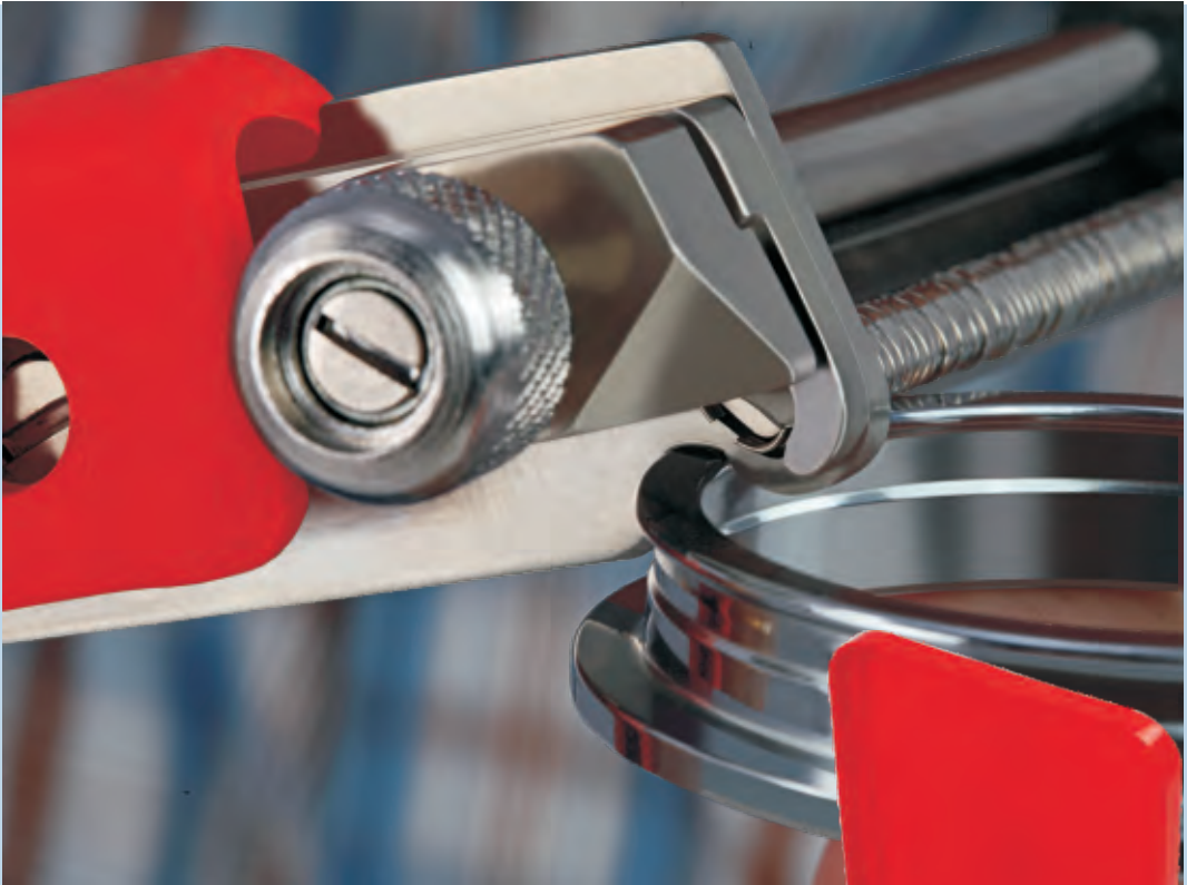
TRAVELLER BEING INSERTED BY AN INSERTING TOOL
