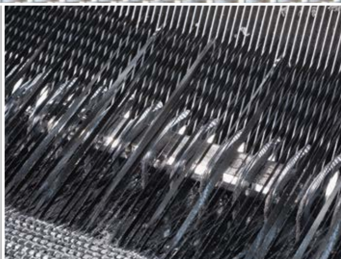
Projectile Weft Insertion: Reliable and Controlled
