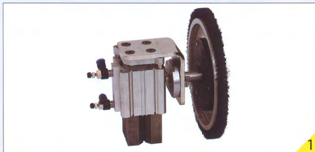
被动毛刷装置 Passive brushing device
