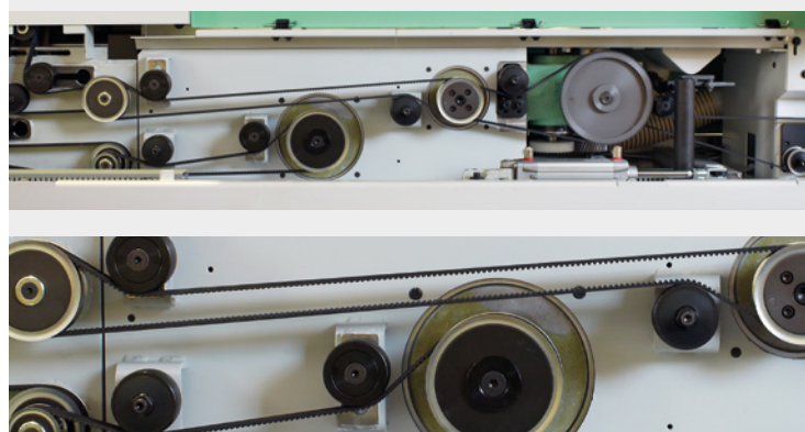
Simple and reliable Toothed Belts Drive System.
