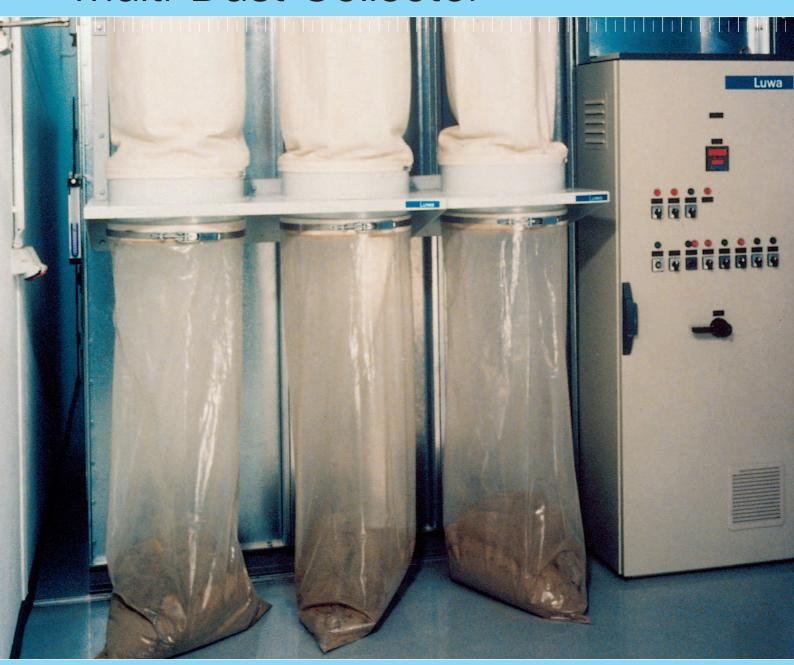
Flexible and simple dust collector group for the disposal of filter waste
