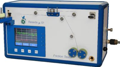
Measurable and practical success: on the newly developed friction tester, the friction levels are measured electronically and evaluated without a separate PC.
