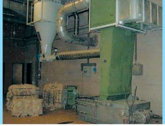
The waste arriving from the dust separator can be collected in a waste bag. By means of the attached screw compactor, the waste is compacted and can be collected in a container or conveyed to a waste press.
