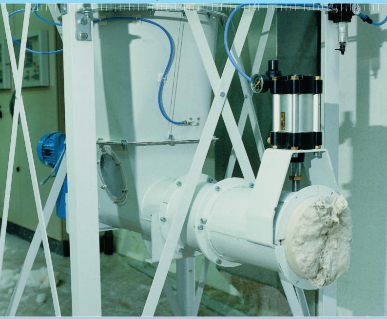
Fully automatic final filtering stage for dust and fibres with discharge and compacting of waste
