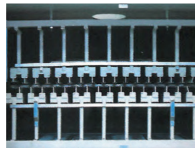
Nozzles with large volumes of air enable the water to be heated very quickly to the evaporation point.
