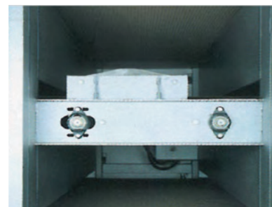
Prior to the drying chamber, the fabric passes through a steam and vibration section, which helps to enhance the fabric volume and soft handle.
